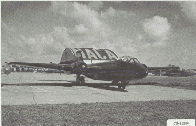
Figure I-6. - B-57 aircraft fueled with hydrogen.
